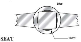
The MK Butterfly Valve seat is constructed by bonding a resilient elastomer to a rigid back-up ring, which forms the outside periphery of the seat. Slip fitted in the valve body, the seat is **field replaceable** without special tools. In the closed position, the disc rim and stem seal lands form an uninterrupted line of sealing contact with the resilient seat, to assure **drop tight sealing** at rated shutoff pressure. MKP seats is offered in a wide range of materials.
